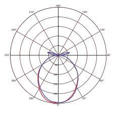
b C0 Plane beam angle(50%) b C90 Plane beam angle(50%) C0 Plane beam angle(50%):102.1(DEG) C90 Plane beam angle(50%):101.4(DEG) Product&Family Code:
