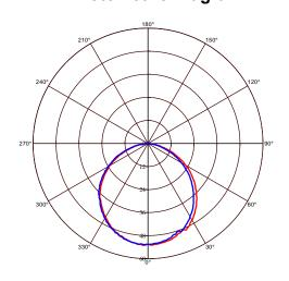
C0 Plane beam angle(50%):110.4(DEG) C90 Plane beam angle(50%):109.6(DEG)
