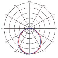
b C0 Plane beam angle(50%) b C90 Plane beam angle(50%) C0 Plane beam angle(50%):105.3(DEG) C90 Plane beam angle(50%):105.5(DEG)
