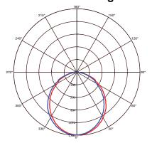
C0 Plane beam angle(50%):105.3(DEG) C90 Plane beam angle(50%):105.5(DEG)
