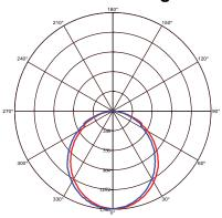
C0 Plane beam angle(50%):105.3(DEG) C90 Plane beam angle(50%):105.5(DEG)
