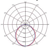
am angle(50%):105.3(DEG) C90 Plane beam angle(50%):105.5(DEG)
