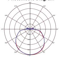
C0 Plane beam angle(50%):137.3(DEG) C90 Plane beam angle(50%):138.8(DEG)
